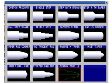
The Unison Motion Control utilizes a Windows 10™ Operating System along with Unison's software to monitor all critical machine functions and alerts the operator to any errors encountered during grinding. Error's are tracked and logged within the machine's Control to easily diagnose the problem. Designed with the machine operator in mind, Unison's "Geometral" software allows for quick customization of any program with minimal effort by just "filling-in-the-blanks".
